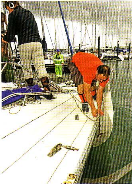
Fothering a sail took a long time and any sail is fundamentally ill-suited for the job
